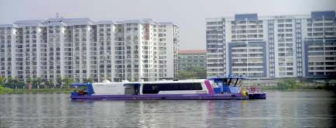
CSL delivered battery operated passenger ferry for the Kochi Water Metro Project to Kochi Metro Rail Limited
